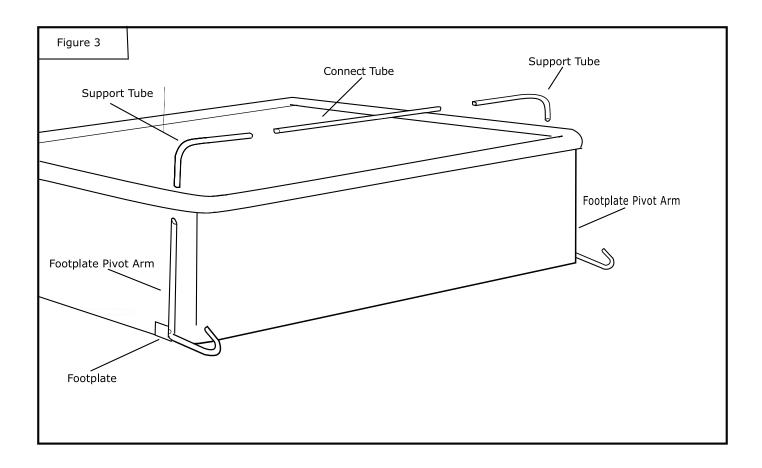
**Step 4:** Lay the Connect tube in the center of the closed spa cover. Depending on your spa size; you must adjust the (2) Support tubes and the (1) Connect tube lengths so they overlap. (per directions in step 6) The Support tubes must be ½" away from the edge of your spa for clearance. Otherwise the lifter may rub on your cabinet. (Fig. 3)
