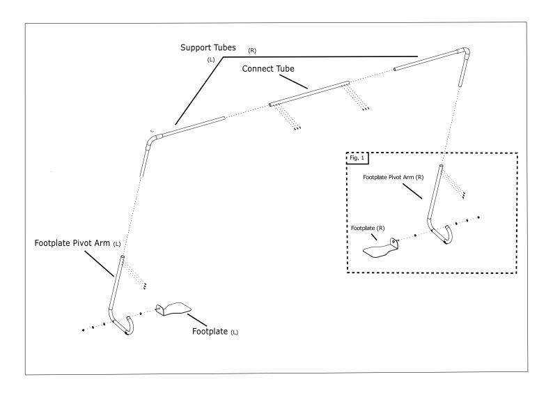
**Components:** (2) Footplates with welded bolts [(1) right footplate (1) left footplate]
